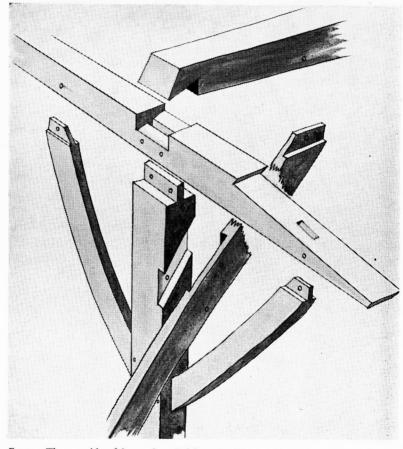
FIG. 5. The assembly of the northern Belchamp Hall barn, as shown also in Fig. 6. Some approach is made in the joints of the tiebeam to a lap-joint form that is able to resist withdrawal, although in this case the resistance is singularly ineffective.
