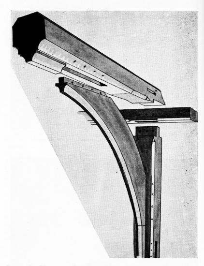
FIG. 12. One tiebeam post and top-plate connection of the barn at Mallbrookes Farm, Mountnessing, Essex (not to scale).
