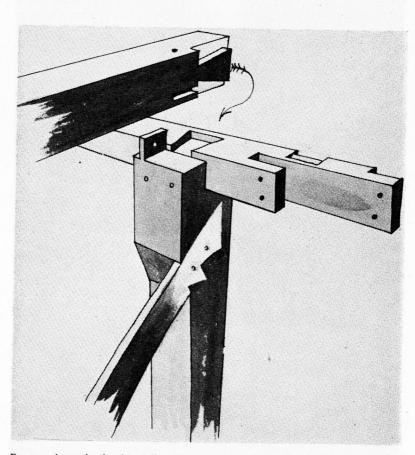
FIG. 17. A post-head and jowl from Cressing Temple Granary, 1628. The scarf-jointing of the top-plate is shown on the right. The jowl-tenon, which holds the tiebeam, is here placed to one side in order not to detract from the strength of the dovetail. The rising-brace, of obscure function, exhibits the double dovetail joint.
